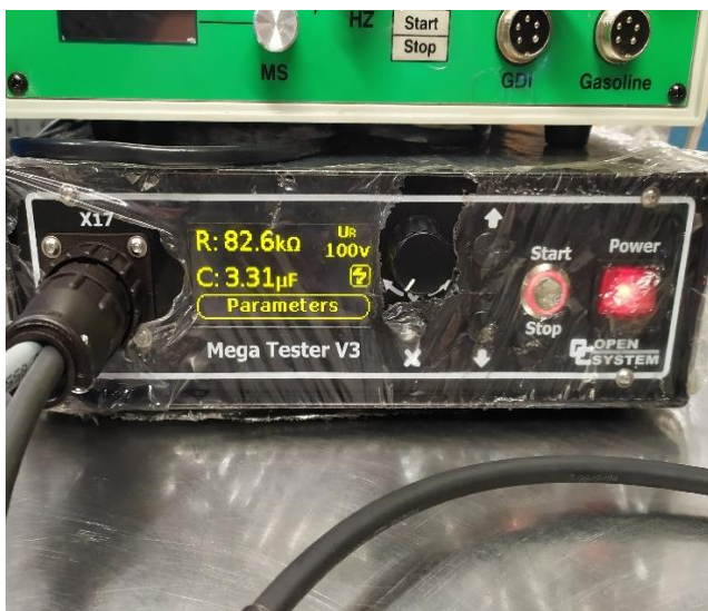
Fig. 4. Failure of the piezoelectric actuator (fuel injector No. 3)
