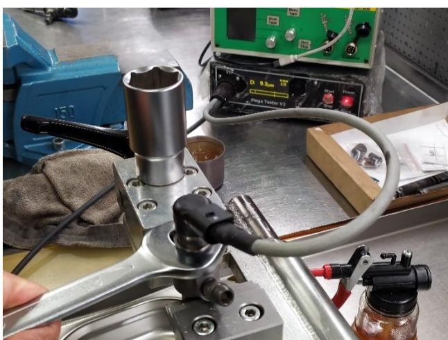
Fig. 9. GAP regulation using the Mega Tester V3 tester
