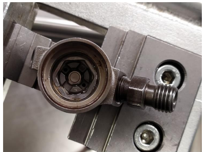
Rys. 6. Fuel injector after disassembling the piezoelectric actuator
