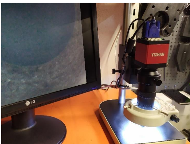
Fig. 8. Examination of the valve seat on a microscope stand
