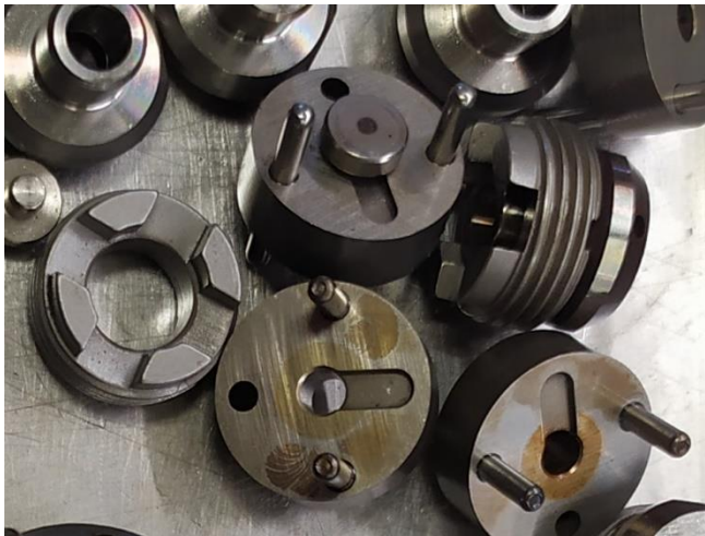
Fig. 7. Disassembled nozzle plunger guides and valve assemblies
