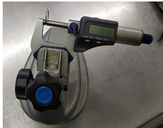
Fig. 10. Measurement of the thickness of the actuator shim
