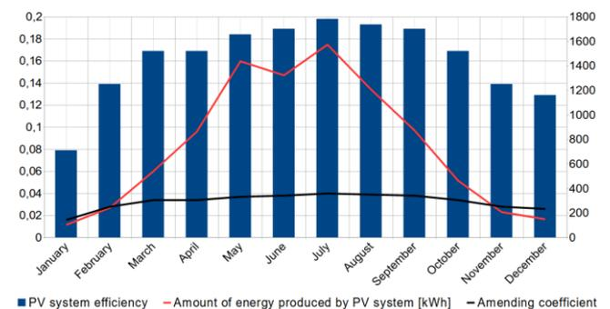
Fig. 3. PV system parameters (numbers at X axis represent months)
