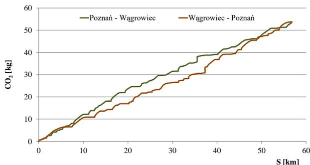
Fig. 6. Total CO<sub>2</sub> emissions during tests in cycles A (Poznań–Wągrowiec) and B (Wągrowiec–Poznań)
