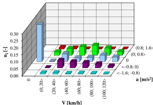
Fig. 4. Shares of research object work time in the speed and acceleration ranges during tests in cycle A
