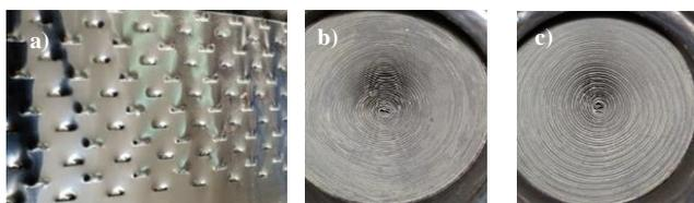
Fig. 7. Prototype filter: a) perforations of metal sheet, b) filter inlet, c) filter outlet
