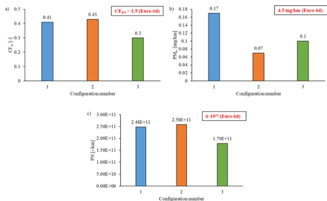
Fig. 20. Summary of the results obtained for each configuration: a) CF<sub>PN</sub>, b) PM<sub>m</sub>, c) PN
