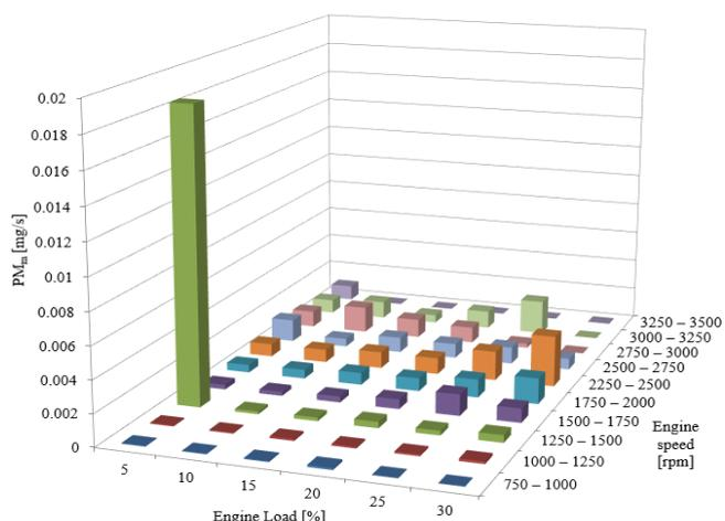
Fig. 18. PM<sub>m</sub> emission intensity in the range of engine speed and engine load for configuration 3 of the exhaust system in the rendered test
