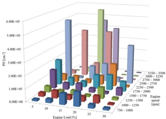
Fig. 16. PN concentration in the range of engine speed and engine load for configuration 2 of the exhaust system in the rendered test
