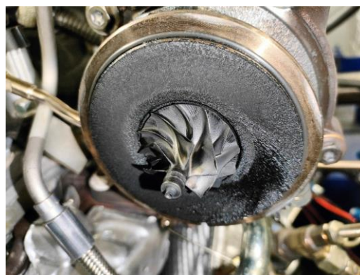
Fig. 24. Contaminated compressor housing after the durability test
