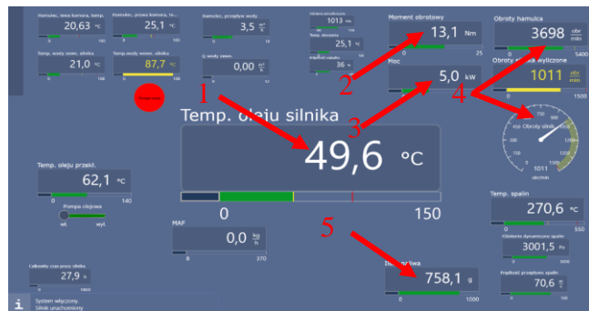
Fig. 3. Single-cylinder engine stand control panel: 1 – oil temperature, 2 – torque, 3 – engine power, 4 – rotation speed, 5 – mass of fuel in the tank
