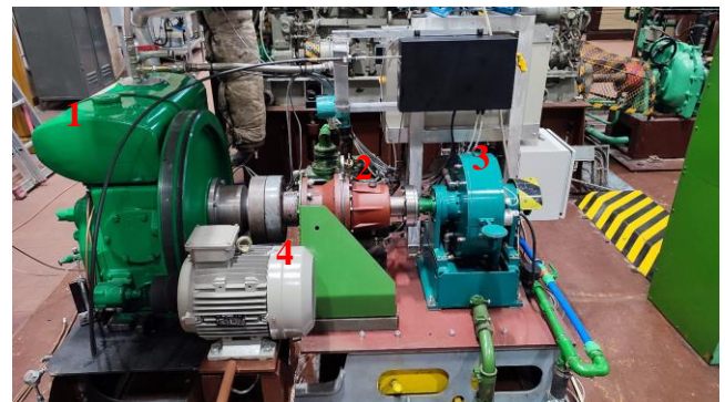
Fig. 2. Laboratory engine station: 1 – engine, 2 – planetary gear, 3 – brake, 4 – electric starter
