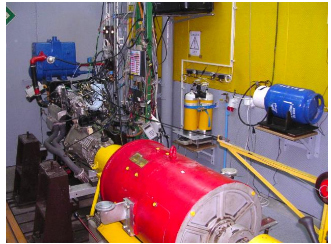
Fig. 2. Test stand with electric brake
