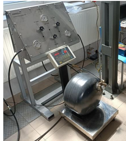
Fig. 3. Station for producing fuel blends
