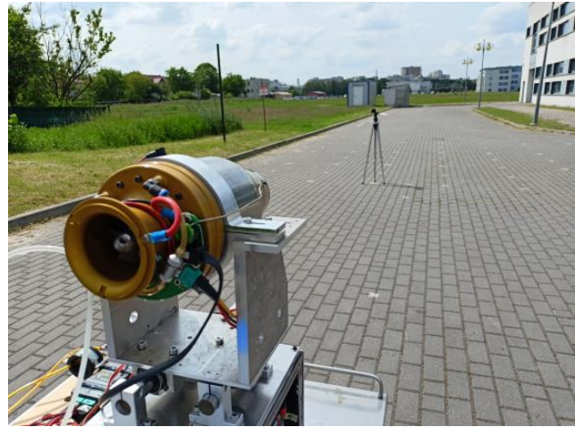
Fig. 6. GTM-120 turbojet at an open space test area
