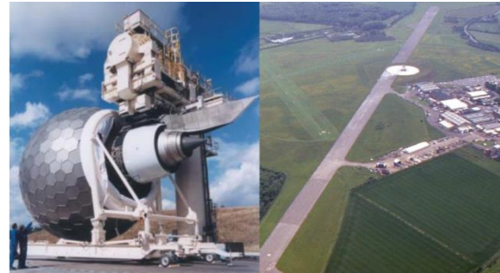
Fig. 3. RR Trent on a test stand no.11 equipped with a TCS system [2]
