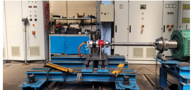
Fig. 8. The tested motor coupled with a planetary gearbox mounted on the torque transducer
