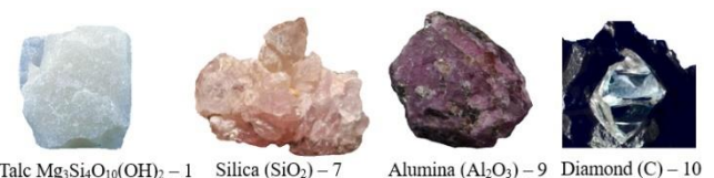
Fig. 23. The form of selected minerals and their corresponding hardness on the Mohs scale [67]
