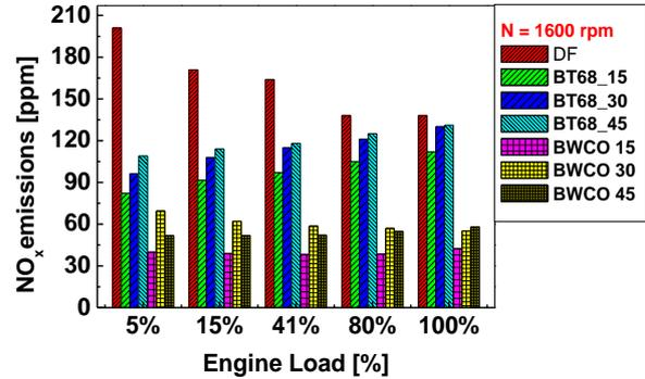
Fig. 9. NO<sub>x</sub> emissions for different biodiesel/diesel blends at different loads
