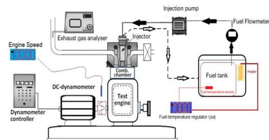
Fig. 4. Schematic view of engine set-up
