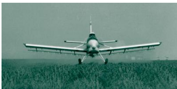
Fig. 1. Kruk Turbo over corn field at very low altitude to make the spraying effective [2]
